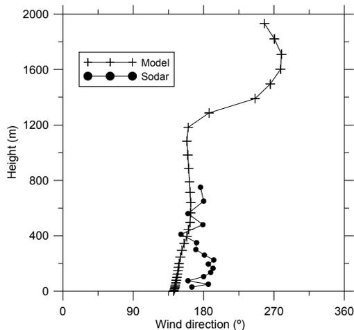
In this figure you can see the comparison between wind profiles measured by Doppler Sodar and modelled with MM5
