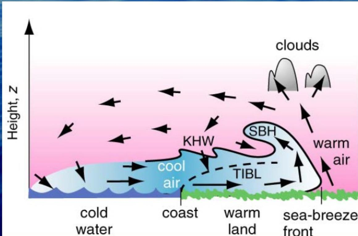
The main idealized components of a mature sea-breeze circulation: SBH = the sea-breeze head, KHW = Kelvin-Helmholtz waves close the head region in the interface between the sea-breeze and return flow, and the thermal internal boundary layer (TIBL), dashed line shows the top. (Wallace and Hobbs, 2006, figure 9.35)
