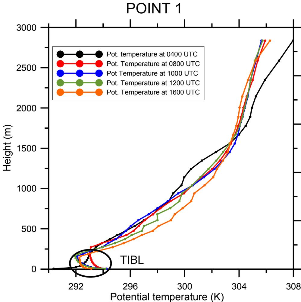
At point 1 the VPPT indicate the formation of a TIBL, which vertical extent is about 250 m.
