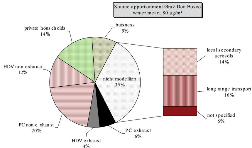
Figure 6. Example of a source apportionment based on the simulations with GRAL for the AQM station Graz-Don Bosco for the winter months in 2006 (Jan-Feb, Dec).
