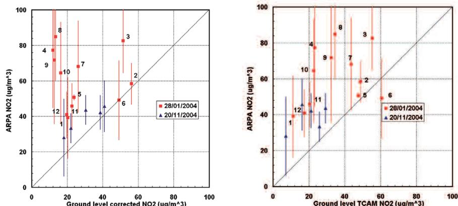
Figure 3. Comparison between ARPA ground measurements (averages of 3 measurements at least with respective variance) and  $GLC_{NO_2}$  for November 20<sup>th</sup> and January 28<sup>th</sup> on the left. On the right we report the same scatter plot but with only TCAM ground level  $NO_2$  concentration (no merging with SCIAMACHY data is performed). The numbers associated with red squares series match with the location of relative SCIAMACHY ground pixel in the first row of Figure 2.
