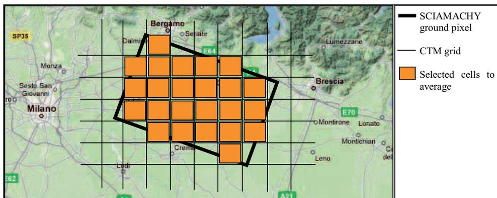
Figure 1. At each overpass all the TCAM simulations whose latitude and longitude match the satellite ground pixel area (orange squares) are considered to calculate and average  $\text{NO}_2$  column from the model ( $C_M$ ).
