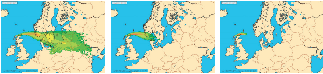
Figure 2. Accumulated total deposition for class 4 (left), 5 (middle) and 6 (right) of the particle radius, 60 hours after explosion.
