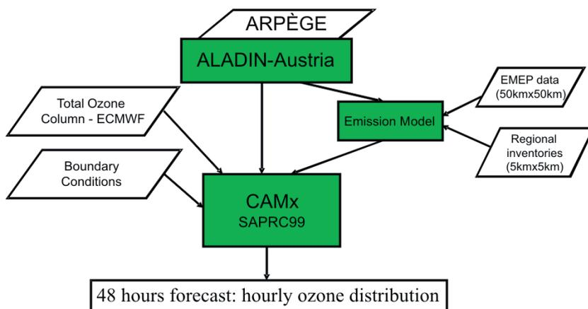
Figure 1. ALADIN-CAMx – air quality modelling system.
