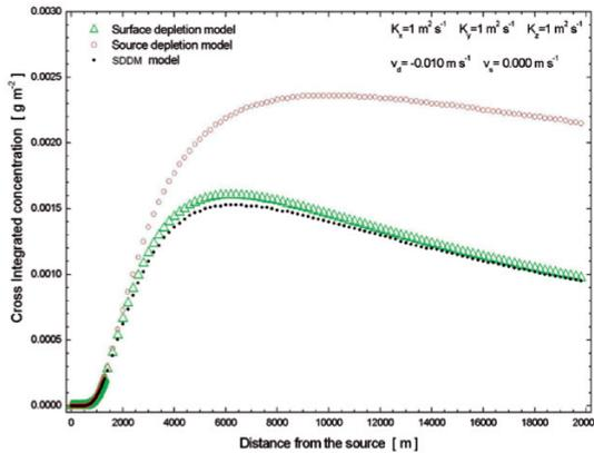
Figure 1. CIC at a ground level for the three models with  $v_d = -0.010 \text{ ms}^{-1}$  and  $v_s = 0.0 \text{ ms}^{-1}$
