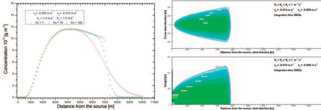
Figure 3. Left: ground level concentration above the plume center line for different  $K_x$ . Right-upper: ground level concentration. Right-lower  $(x,z)$  at the plume center line direction.
