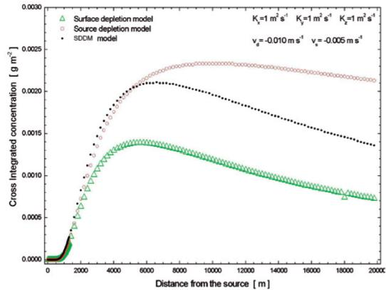
Figure 2. CIC at a ground level for the three models with  $v_d = -0.010 \text{ ms}^{-1}$  and  $v_s = -0.005 \text{ ms}^{-1}$
