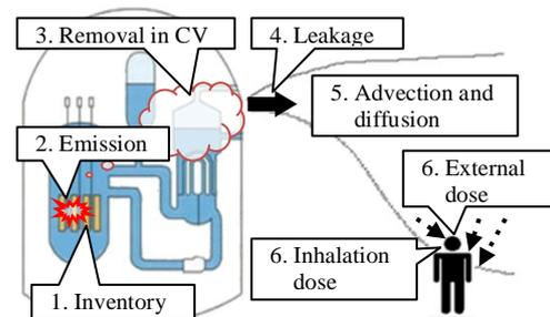
Figure 1. Procedure to predict release amount and dose
