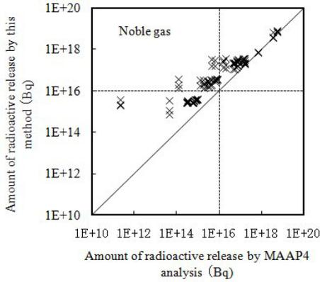
Figure 2. Comparison of noble gas 0.5MeV equivalent release amounts between MAAP4 and this model
