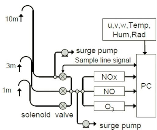
Figure 1. Sampling line and measurement system.
