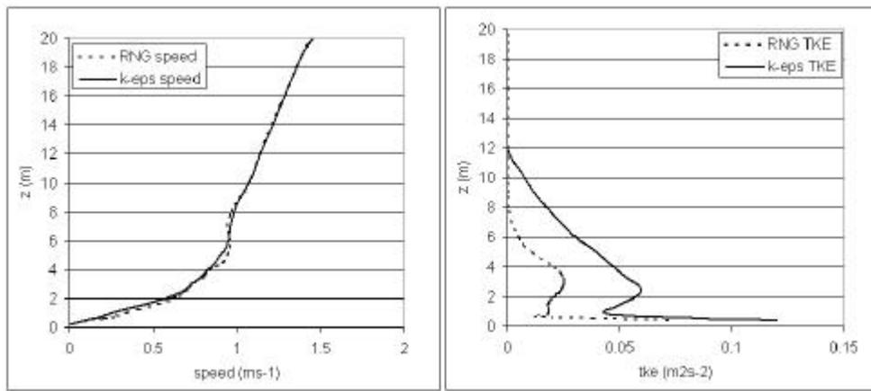
Fig. 4; Wind speed (left) and tke (right) profiles at the domain's centre ( $x=0.4$  m,  $y=0.6$  m)
