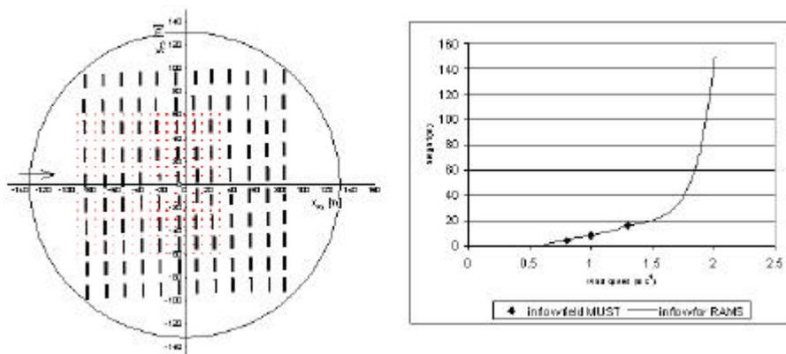
Fig. 1; Geometry of 0° inflow MUST field experiment (courtesy of B. Leitl), left, and wind profile for RAMS simulation initialisation in MUST field test case, right.
