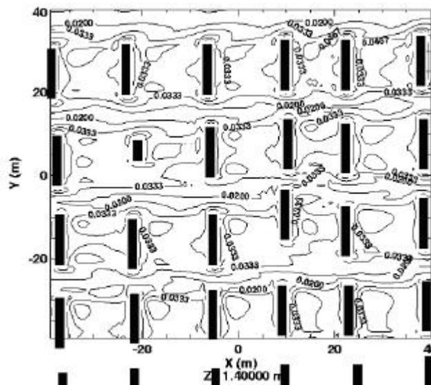
Fig. 3; Difference in turbulent kinetic energy field between  $k-\epsilon$  and RNG  $k-\epsilon$  simulations.
