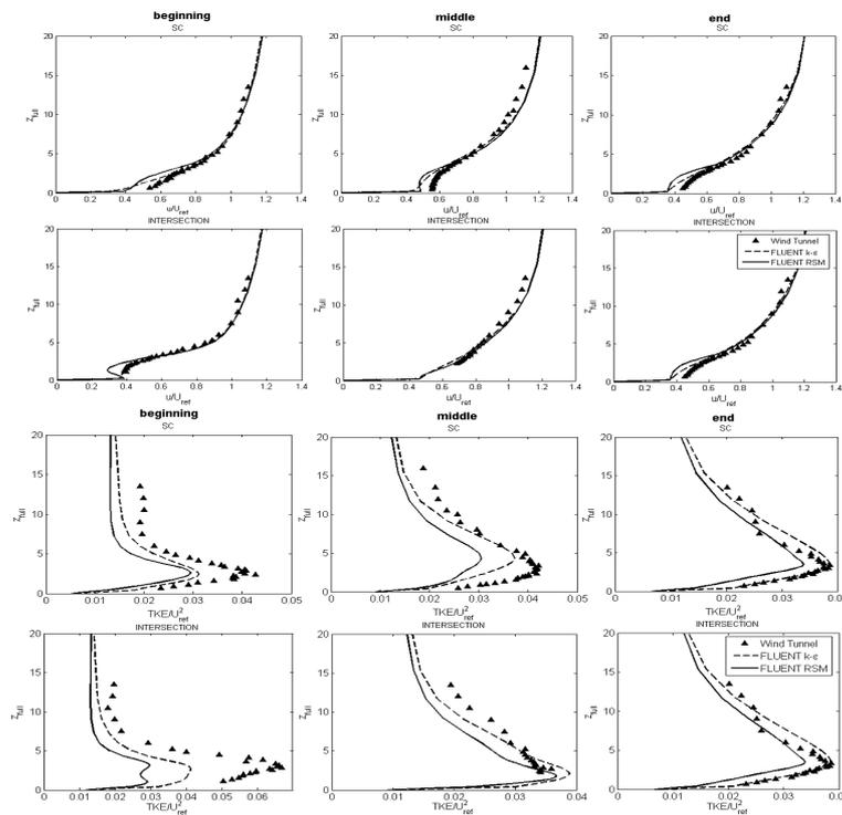
Fig. 3; -45° approaching flow case: vertical profiles of  $u/U_{ref}$  (top) and  $TKE/U_{ref}^2$  (bottom).
