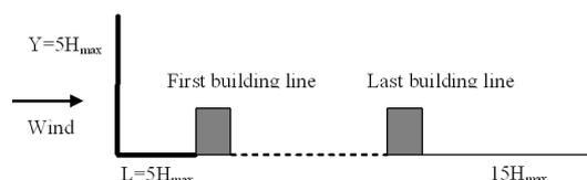
Fig. 1; Schematic view of the extent characteristics of the computational domain used.
