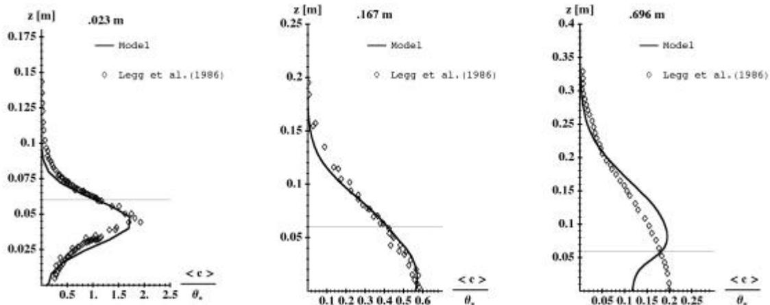
Fig. 1; Mean concentration normalized with the concentration scale  $q_*$  (Legg et al., 1986). The horizontal line represents the canopy height. The number at the top of each figure is the distance from the source.
