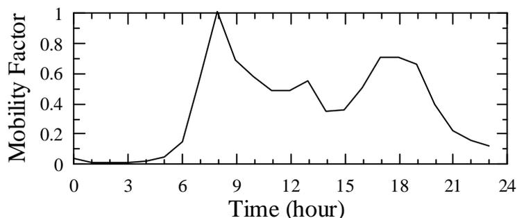
Fig. 2; Mobility factor for a typical working day in the city of Rome.
