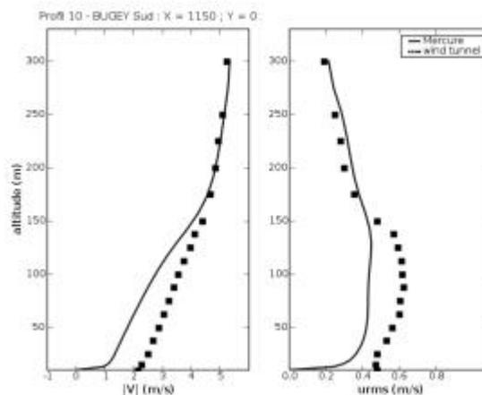
Fig. 3; Vertical profile of wind magnitude and rms longitudinal wind fluctuation predicted by CFD Mercure\_Saturne and wind-tunnel experiment located 350 m behind the cooling towers, where the differences are maximum.
