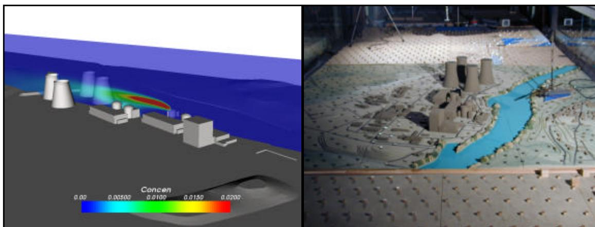
Fig. 1; Left: Mercure\_Saturne modelling of the stack release. Right: experimental model.
