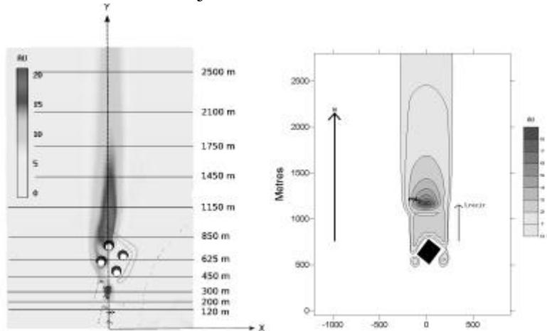
Fig. 4; Predicted ground level concentration in arbitrary units for the stack release, respectively for Mercure\_Saturne (left) and ADMS (right).
