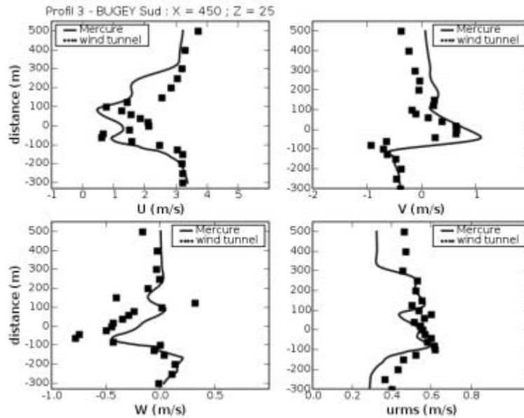
Fig. 2; Cross-wind profile of wind components and rms longitudinal wind fluctuation predicted by CFD Mercure\_Saturne and wind-tunnel experiment at the level  $z = 25$  m, located just upstream of the first cooling tower.
