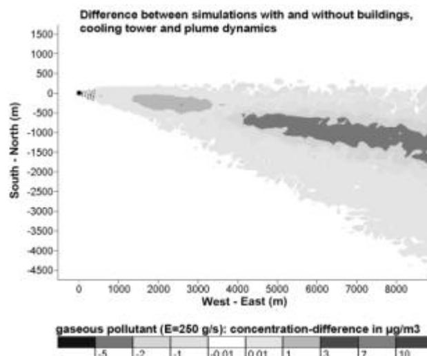
Fig. 5: Difference in surface concentration between simulation with buildings, cooling tower and plume dynamics and a calculation without those effects. Explanation see text.
