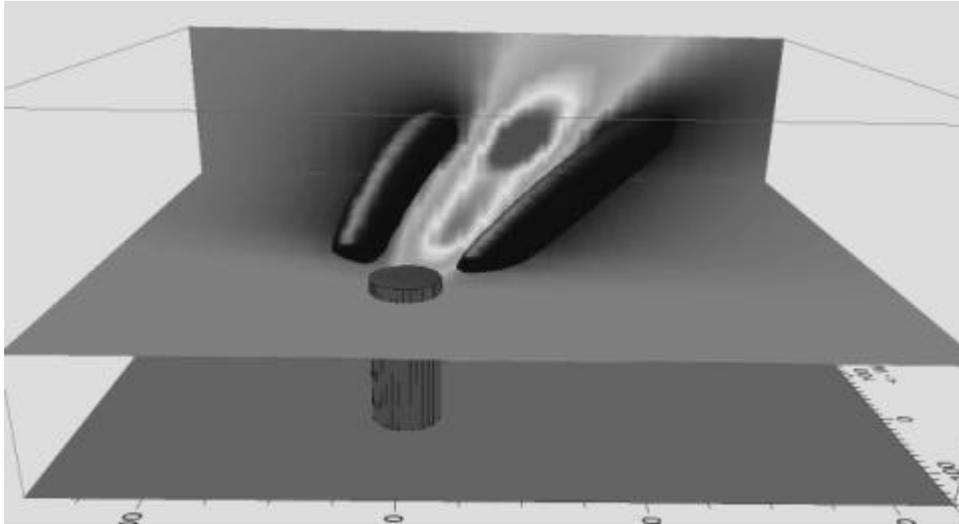
*Fig. 3: Downwind view of the flow structure of water-vapour plume of a cooling tower. Dark “tubes”: Downdraft areas. Horizontal and vertical cross-sections show the updraft at the centre of the plume. Result of wind field modelling with added counter-rotating vortices.*
