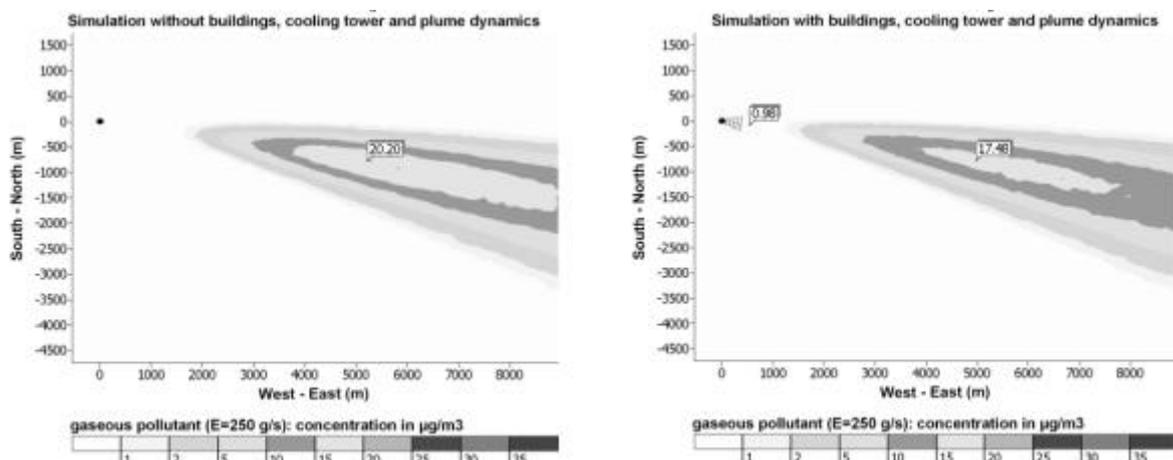
Fig. 4: Surface concentration field of simulation without any buildings and without plume dynamics (left) and with explicit consideration of both effects in wind field and dispersion calculation (right).
