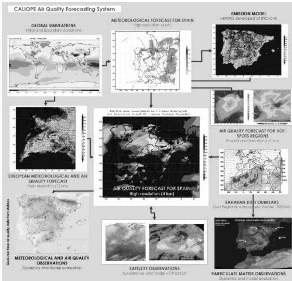
Fig. 2; Structure of the air quality forecasting system of the project CALIOPE implemented in MareNostrum supercomputer.
