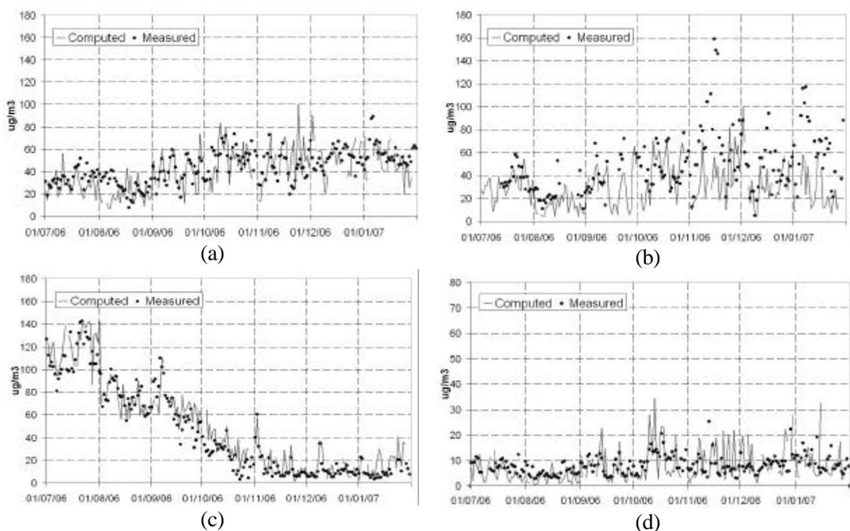
Fig. 5; Comparison between measured and computed daily average ground concentration levels. (a)  $NO_2$  concentrations, Novara – Via Leonardi monitoring site (b)  $PM_{10}$  concentrations, Novara – Via Verdi (c)  $O_3$  concentrations, Novara – Via Verdi (d)  $SO_2$  concentrations, Novara – Via Bovio.
