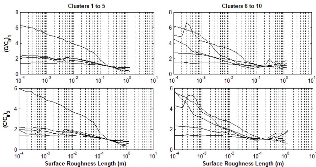
Fig. 3; Sensitivity of AERMOD to changes in Surface Roughness Length. The upper diagrams refer to the maximum concentrations normalized by the maximum concentration of the base case  $C_0$ , while the lower ones correspond to the second maximum estimated concentrations.
