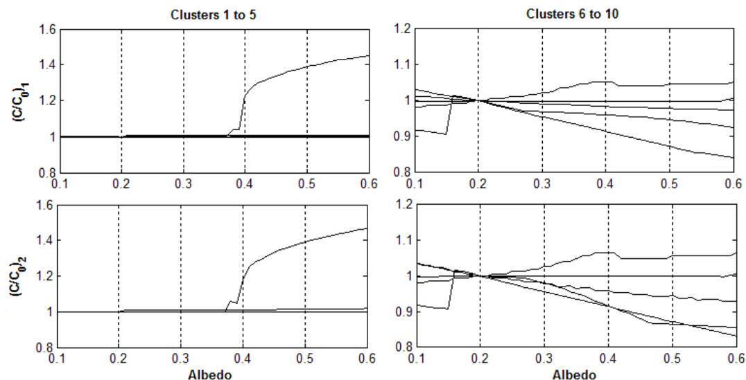
Fig. 3; Sensitivity of AERMOD to changes in Albedo.
