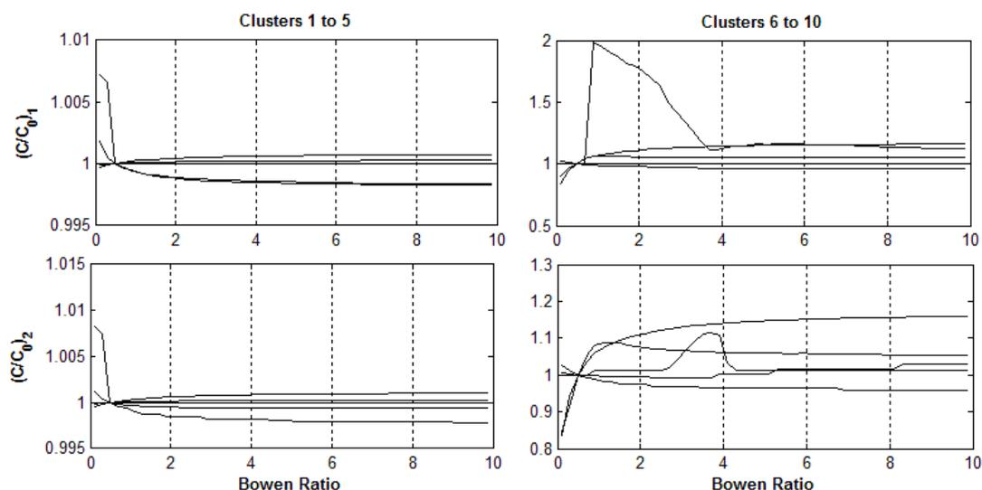
Fig. 5; Sensitivity of AERMOD to changes in Bowen Ratio.
