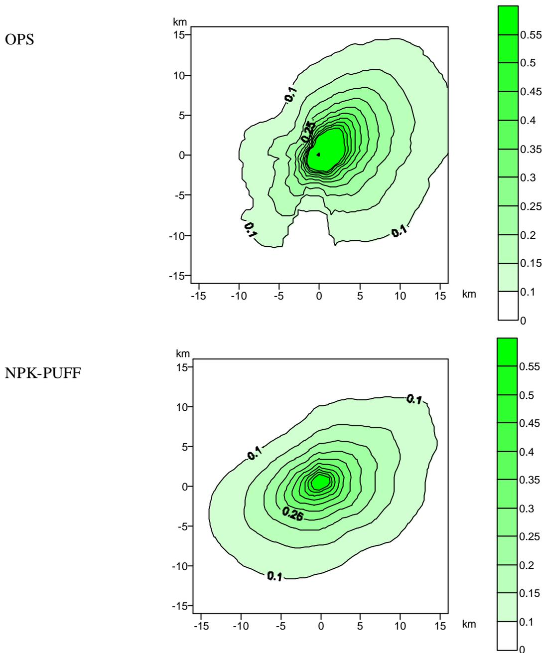
Fig. 1; Concentration in air (in mBq/m<sup>3</sup>) from the continuous emission, over the year 2005, of 500 GBq of the polonium isotope <sup>210</sup>Po: OPS model (top) and NPK-PUFF model (bottom). The distance between receptors is 0.5 km. This comparison shows auspicious agreement.
