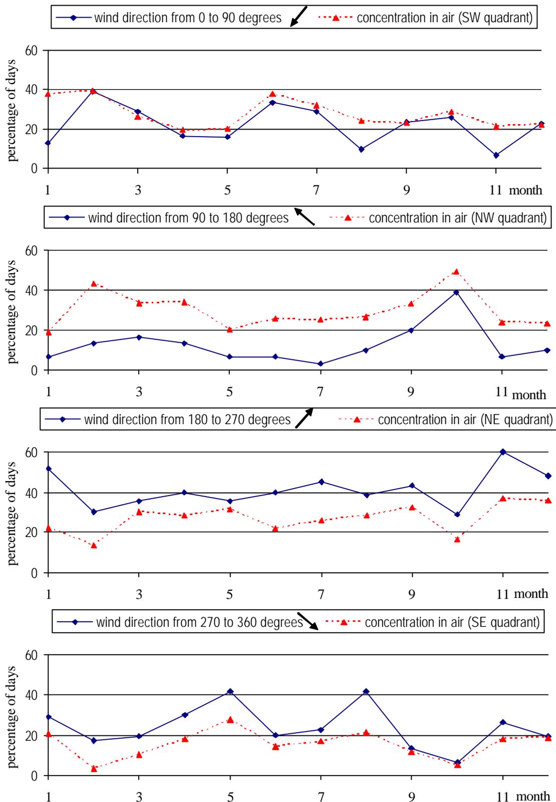
Fig. 2; Correlation between wind direction and modelled contaminant concentration in air. Within the grid calculation field of NPK-PUFF, the monthly sum of the contaminant concentration in air in the four quadrants is shown (normalized to the total in the calculation grid), together with the percentage of days for each month in 2005 when the wind blows in the direction of each quadrant. The correlation coefficient varies between 0.56 and 0.85.
