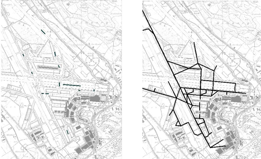
Fig. 3; Monitor versus scenario calculation (Zürich Airport). Left: Snap-shot of aircraft traffic in a monitor calculation, showing the line segments that 12 aircraft pass in the depicted 10-second interval. Right: Stationary line sources for taxiway emissions in a scenario calculation.
