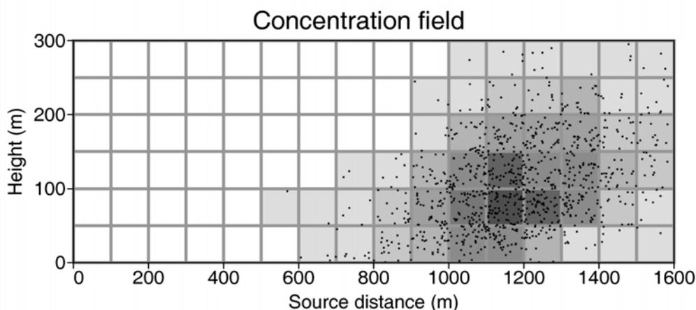
*Fig. 2; Working with particles in a Lagrangian particle model. A vertical intersection of a cloud of simulation particles (black points) from which the concentrations in each cell of a regular grid is derived (encoded here as background colour of each cell).*
