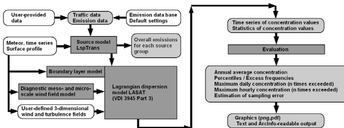
Fig. 1; General structure of the program system LASPORT.
