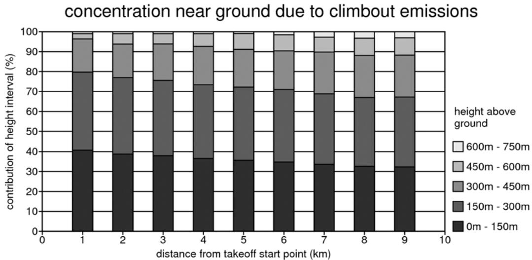
Fig. 4; Sensitivity analyses. Contribution of different height layers to the concentration near ground at 9 monitor points for the climb out emission of a single aircraft (Janicke, U., 2006).
