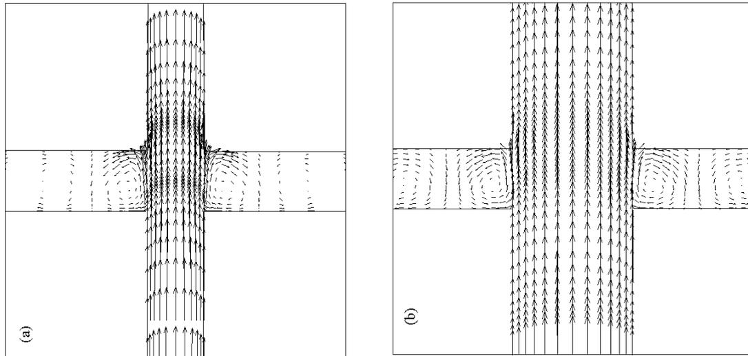
Fig. 2; Mean velocity field in the street intersections at  $z=H/2$ : (a) Conf-1 and (b) Conf-3.
