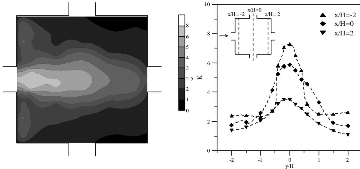
Fig. 7; Mean concentration field at  $z=H/2$  (wind tunnel) and mean concentration transversal profiles
