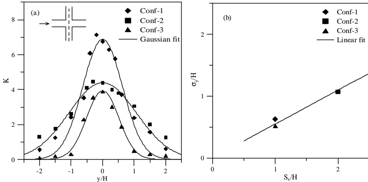
Fig. 4; (a) Transversal mean concentration profiles and (b)  $\sigma_y$  values for the different street intersections
