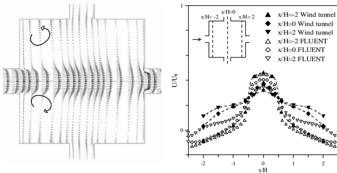
Fig. 5; Mean velocity field at  $z=H/2$  (FLUENT) and mean velocity transversal profiles
