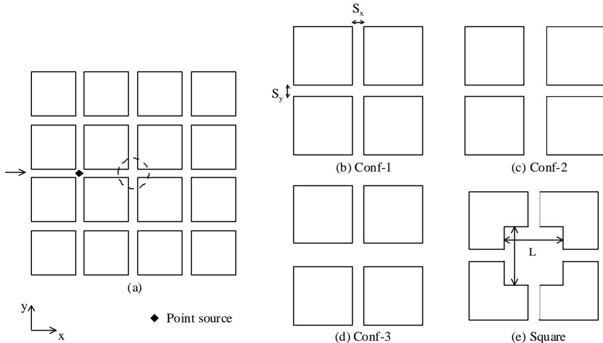
Fig. 1; Wind-tunnel set up and the investigated configurations.
