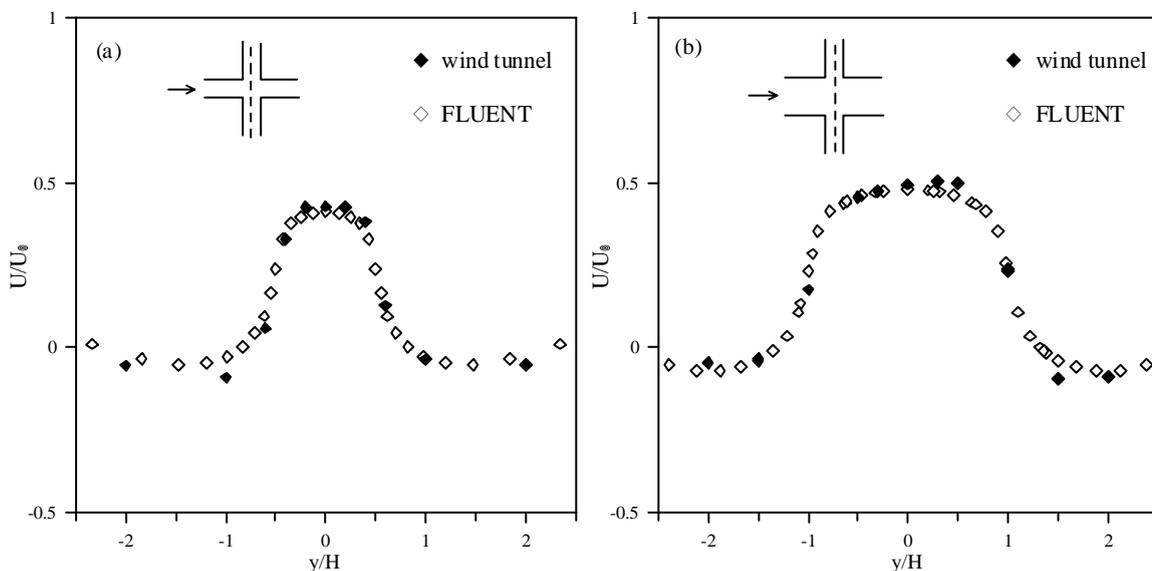
Fig. 3; Mean velocity transversal profiles at  $z=H/2$ : (a) Conf-1 and (b) Conf-3.
