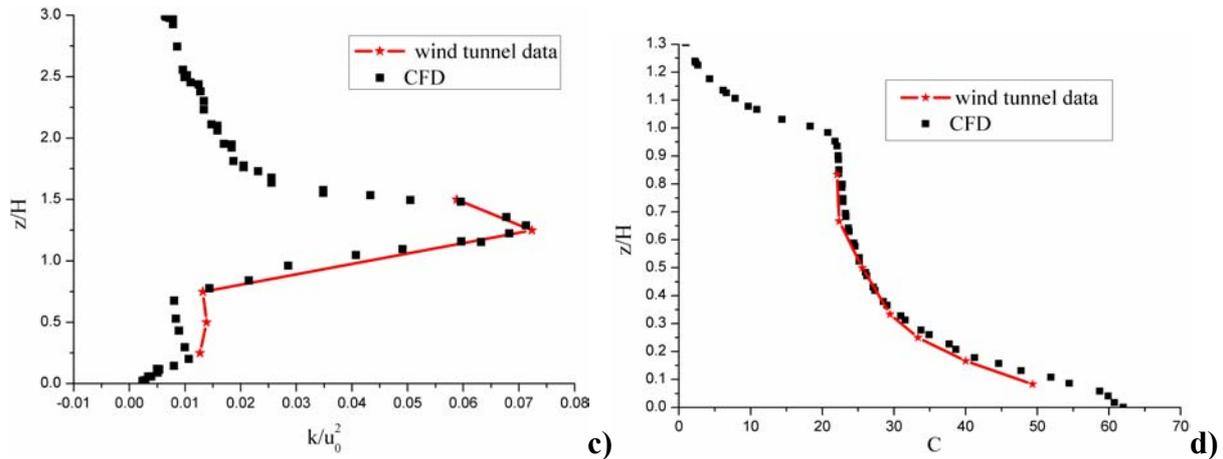
Figure 1. Comparison between wind tunnel data and CFD calculations for mean horizontal (a) and vertical (b) velocity components, TKE (c) and normalised concentration (d).
