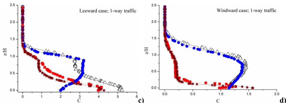
Figure 3. Normalised concentration for 2-way traffic configuration: leeward (a) and windward (b) side, and 1-way traffic configuration: leeward (c) and windward (d) side. Symbols as in (b).
