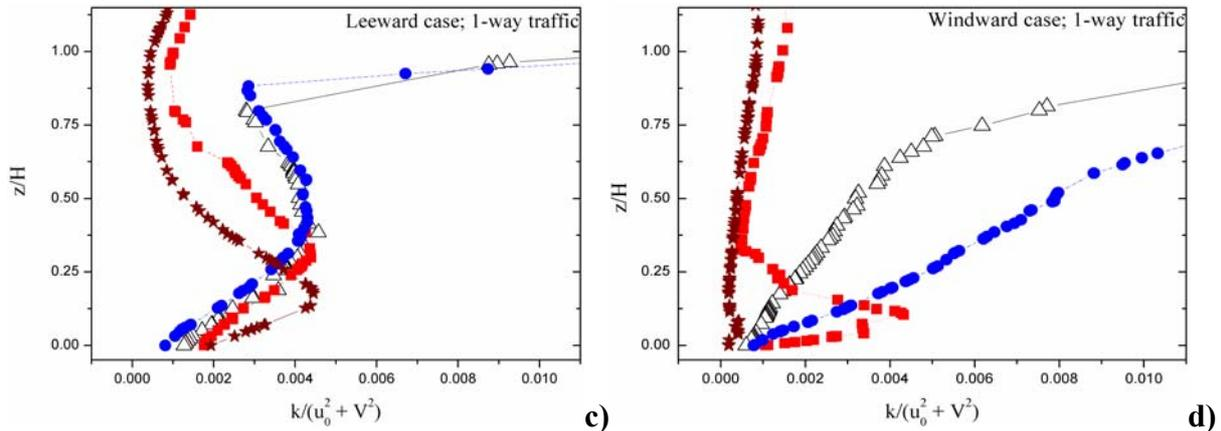
Figure 2. Normalised TKE for 2-way traffic configuration: leeward (a) and windward (b) side, and 1-way traffic configuration: leeward (c) and windward (d) side. Symbols as in (b).
