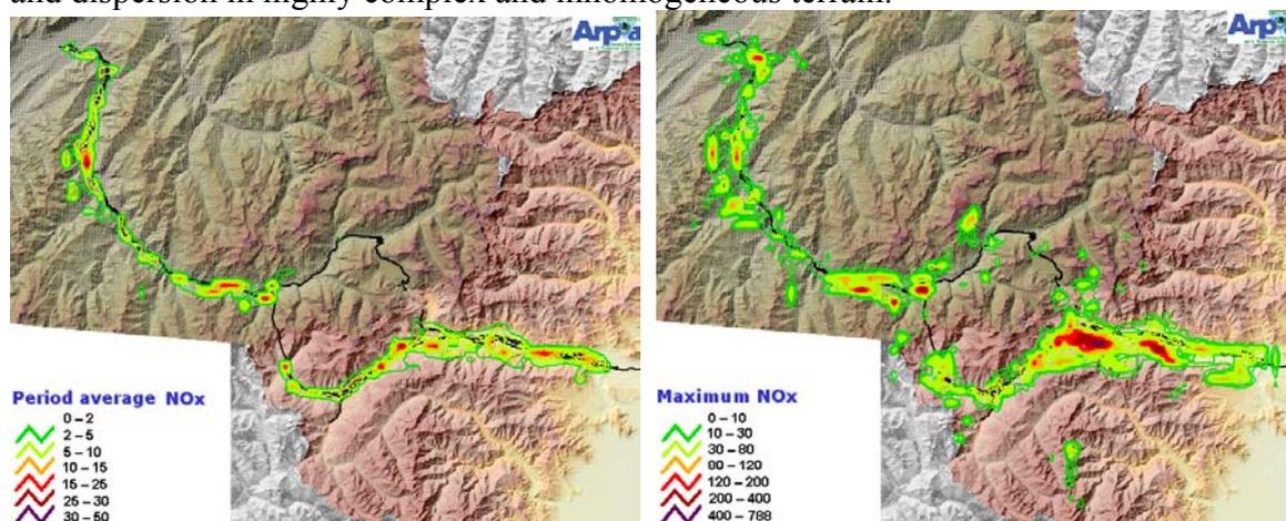
Fig. 5; SPRAY simulation on 1 km resolution domain: mean(left) and maximum(right) NOx concentration field calculated for all period 08-14 February 2004.
