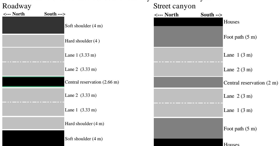
Figure 1: Layouts used in the tests.
