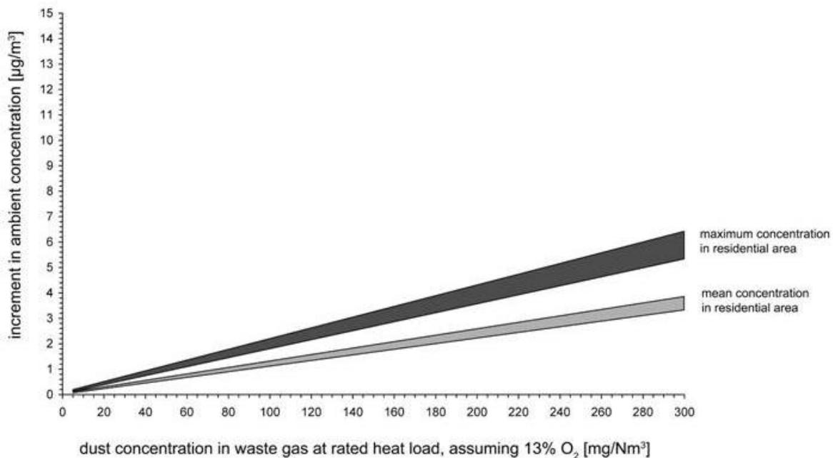
Fig. 3; Contribution of 10 % wood burning boilers to the ambient annual average PM10 concentration in the low-density, rural residential area. Ambient temperatures and winds represent average conditions in Southern Germany.
