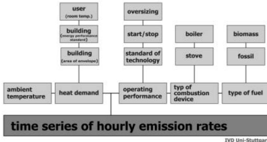
Fig. 2; Emission model (Struschka, M., W. Juschka and G. Baumbach, 2007)
