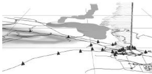
Figure 3 : 3D data and result visualisation: Arrows represent the radiosounding winds, the cloud just after stabilisation, main receptors (monitoring points), long range HCl impact for an Ariane5 launch (A502)
