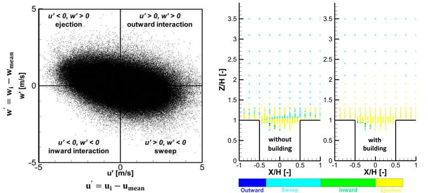
Left: Scheme of the quadrants and scatter plot of the measured velocity fluctuations in a point at  $Z/H=1.1$  (at  $X/H=0$ , without building). Right: distribution of the dominant event in a measurement points at K13 in Plane 3
