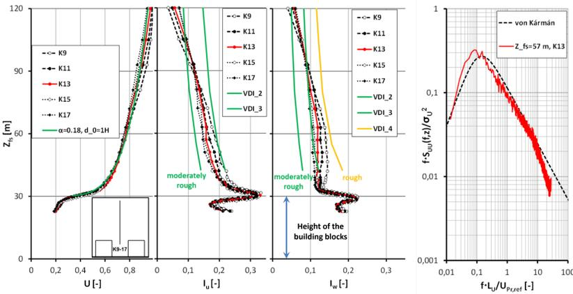
Dimensionless velocity (U), longitudinal ( $I_u$ ) and vertical ( $I_w$ ) turbulent intensity profiles at the centreline of canyons K9-17 (the height above the surface is expressed in full scale, therefore the top of the building blocks are at  $Z_p=30$  m). Left: dimensionless power spectral density of the longitudinal velocity fluctuations at height  $Z_p=57$  m (K13) compared to the theoretical von Kármán spectrum.
