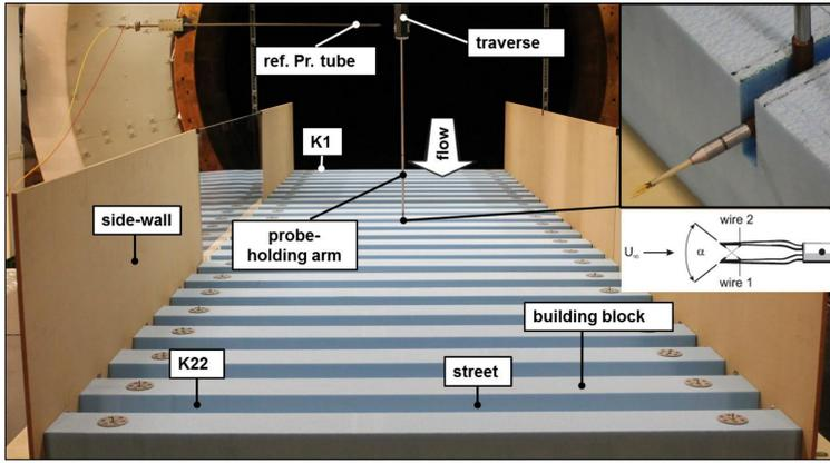
Based on these considerations, wind tunnel model was constructed and placed in to the test section of the Large Wind Tunnel of the Theodore von Kármán Wind Tunnel Laboratory, containing 22 street canyons (K1-K22) with height of 100 mm and width of 1250 mm. The scale of the model was 1:300. The measurements were carried out at reference velocity 10.5-11.5 [m/s].
