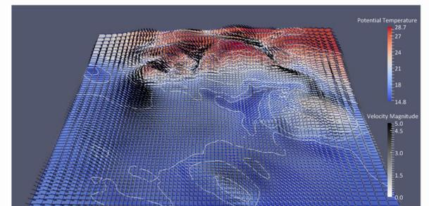
Figure 4: PROWIMO simulation results for Tehran on the D02.1 domain: Ground level wind and potential temperature distribution.
