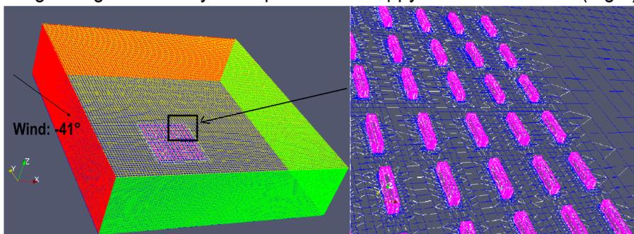
Figure 3: Site features and generating mesh using snappyHexMesh utility
