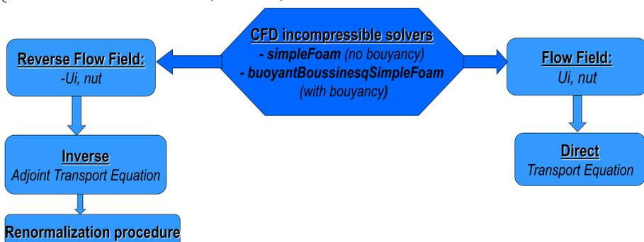
Figure 2: Schematic view of the numerical coupling in the direct and inverse dispersion problem using OpenFoam solvers
