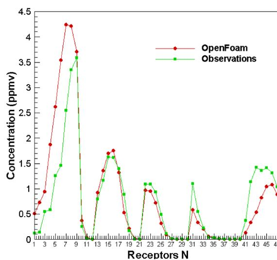
Figure 5: C<sub>3</sub>H<sub>6</sub> concentration (in ppmv) at each sensor
