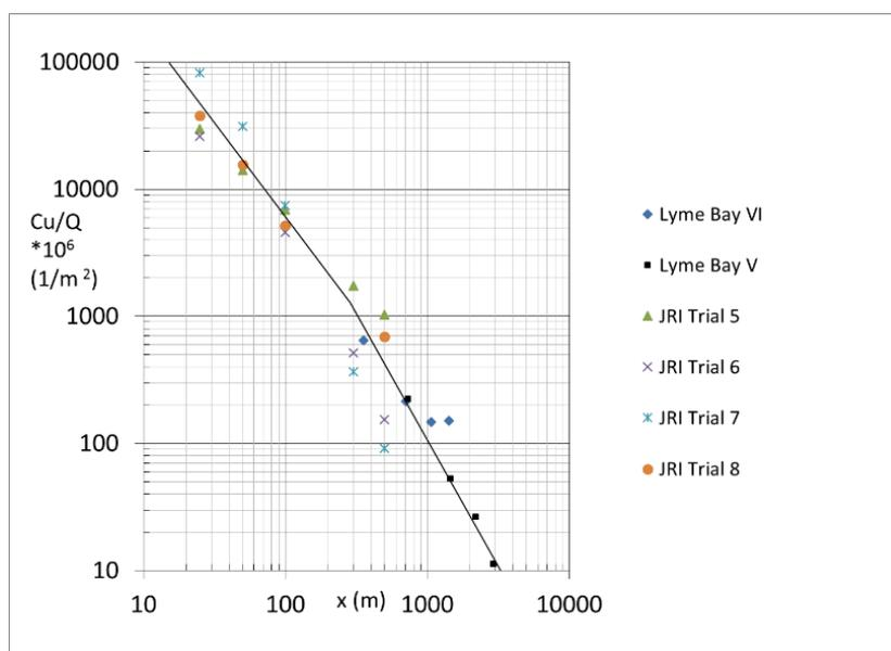
**Figure 1.** Lyme Bay and JR I observed  $\ln C_u/Q_c$  versus  $\ln x$  (from Hanna et al., 2016).  $C$  is one-min avg arc max,  $u$  is wind speed, and  $Q_c$  is mass emission rate.
