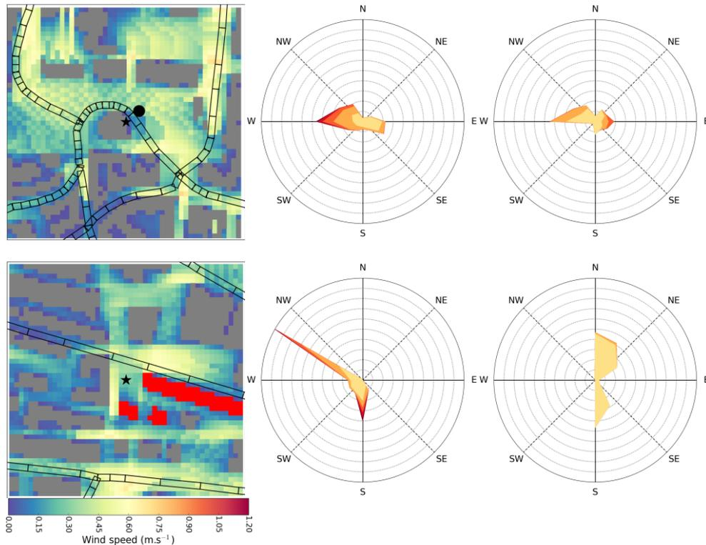
**Figure 1.** Local situation of two observation sites (top: LAU; bottom: DGE07) and observed (left) and simulated (right) wind roses. Observations are located at the black stars. For LAU, the wind measurements (black dot) are slightly shifted compared to the concentration observations (black star).
