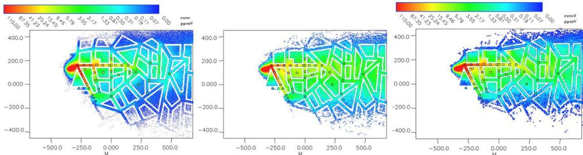
**Figure 2.** Concentration contours in the simulation domain for CONF\_1, CONF\_2 and CONF\_3 (from left to right). The coloured squares represent the observations in the same colour scale as for the simulations.
