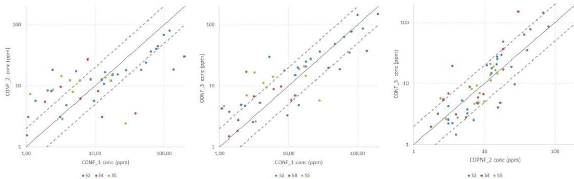
**Figure 3.** Scatter plots (logarithmic scale) of the different setups predicted concentration values at the measuring locations for the release at sources S2 (blue points), S4 (red points) and S5 (green points)
