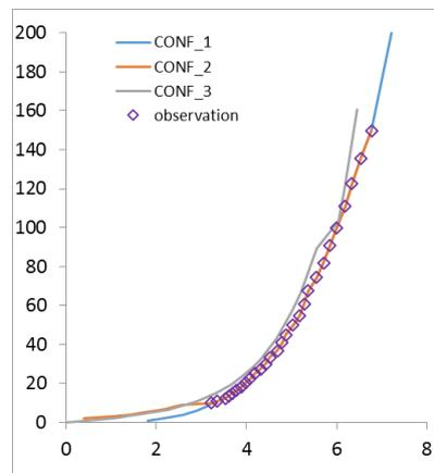
**Figure 1.** Michelstadt case. Inlet wind speed profile as used in the three different configurations (solid lines, blue for ‘CONF\_1’, dark red for ‘CONF\_2’ and green for ‘CONF\_3’) and experimental data (diamonds).
