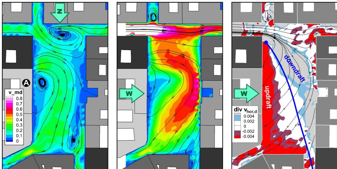
**Figure 5.** Left: LDV flow field results at  $0.5h$  height in the complex square at north wind direction; centre: at west wind; right: calculated vertical velocity using the divergence method. Note the strong helical vortex
