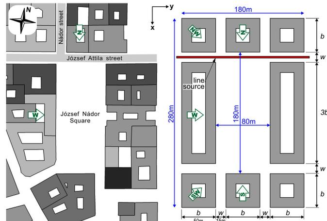
**Figure 1.** The urban square geometries investigated. Buildings are coloured by height. Left: real geometry of József Nádor Square, Budapest; right: simplified square.
