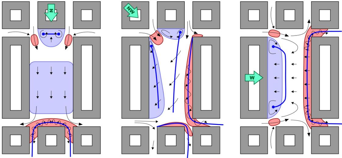
**Figure 4.** The schematic flow fields in the simplified square at various wind directions. Black arrows: pedestrian level wind directions, thick blue lines: vortex cores, purple areas: high wind speed zones near the ground; light blue areas: low wind speed zones near the ground.
