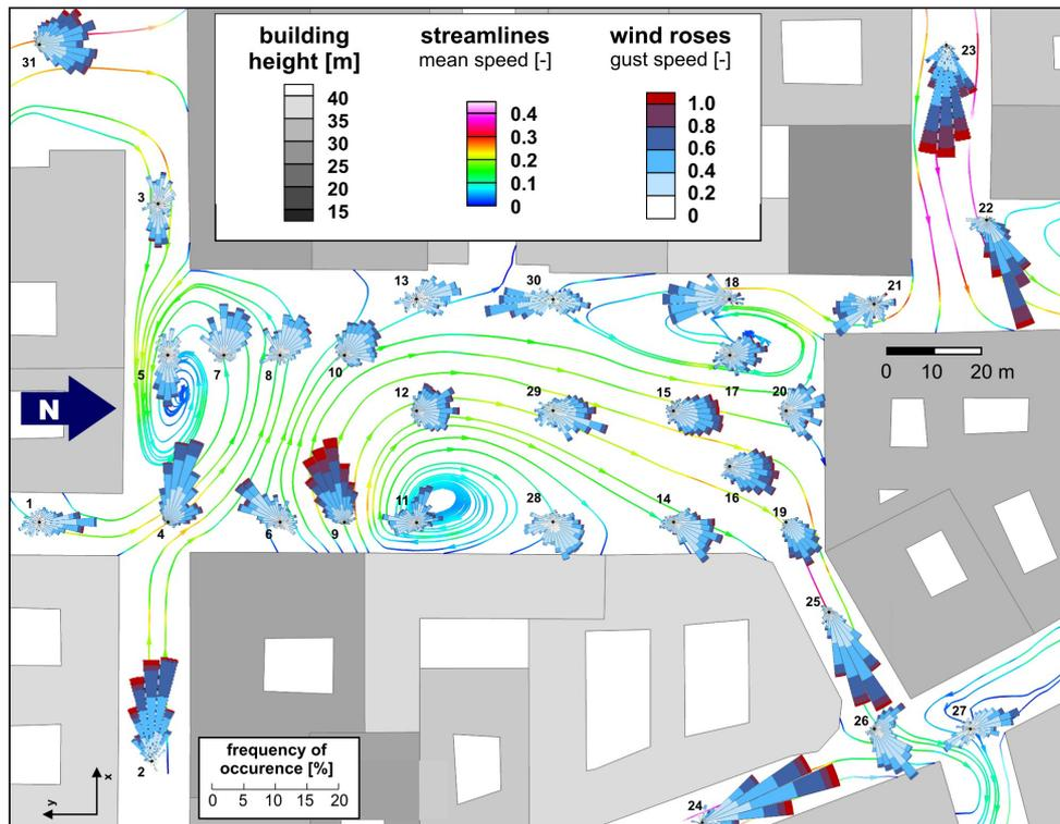
**Figure 7.** Flow field and wind roses at northern wind direction at 0.5 h height. Streamlines are coloured by average velocity magnitude  $v_{md}$ , and wind roses by the magnitude of the instantaneous wind vectors
