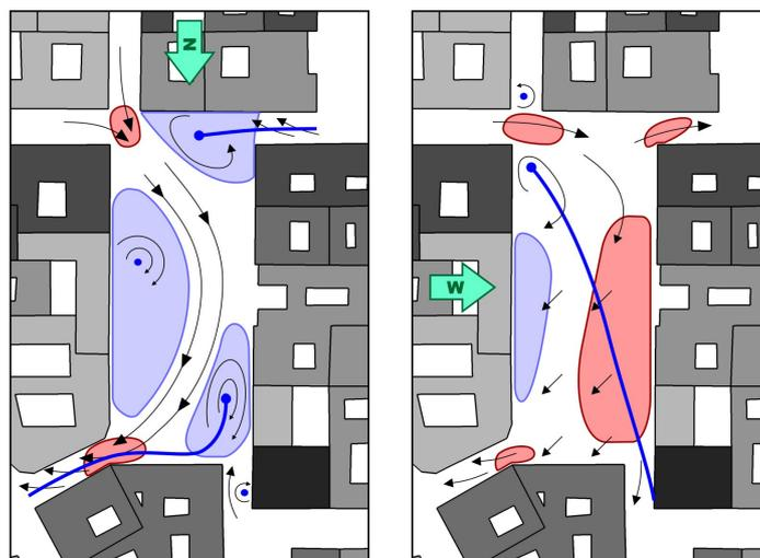
**Figure 6.** The schematic flow fields in the complex urban square at various wind directions
