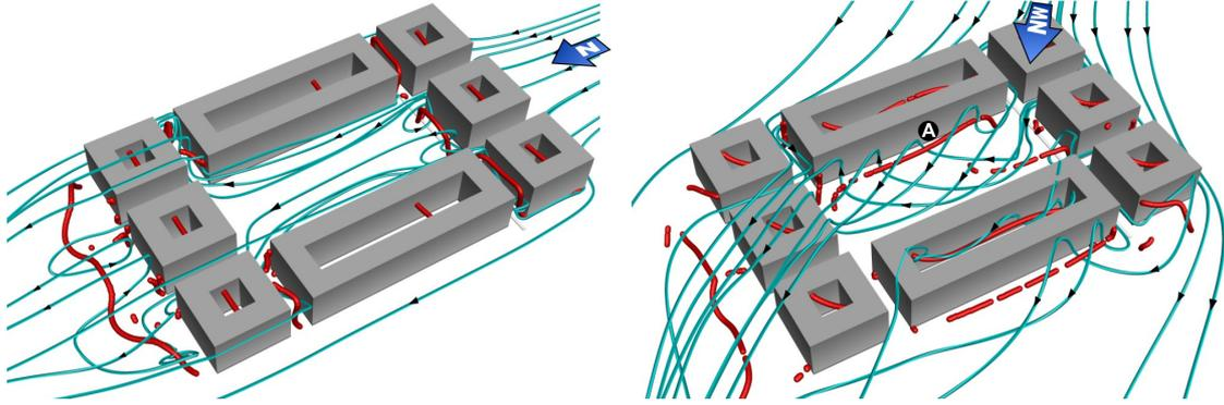
**Figure 3.** Flow structures at north and north-west wind direction. Note the large helical vortex dominating the square at north-western wind (marked by A)
