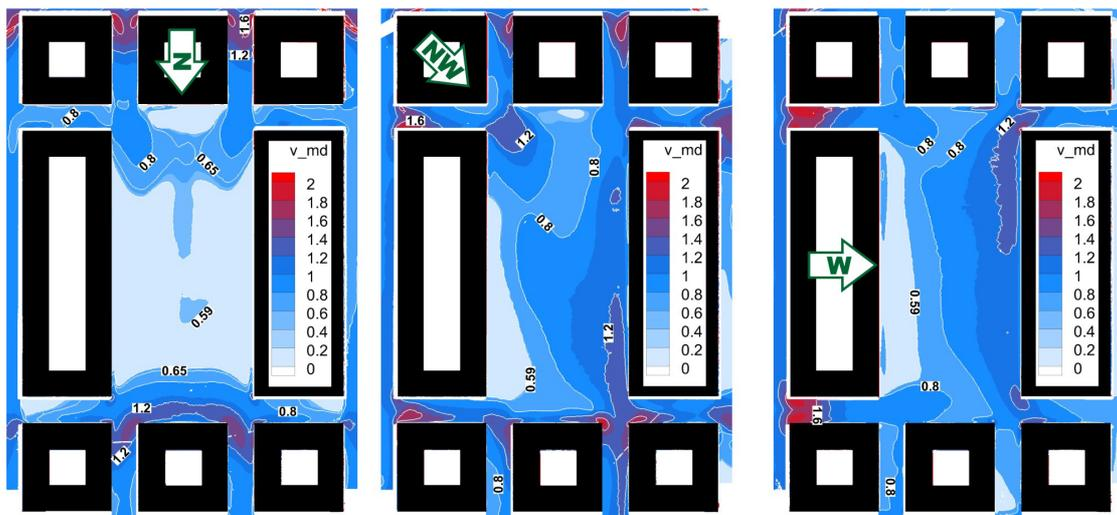
**Figure 2.** Sand erosion results for normalized mean wind speed at various wind directions.
