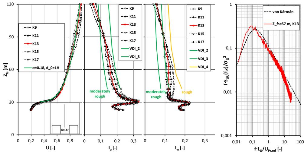
**Figure 2.** Dimensionless velocity ( $U$ ), longitudinal ( $I_u$ ) and vertical ( $I_w$ ) turbulent intensity profiles at the centreline of canyons K9-17 (the height above the surface is expressed in full scale, therefore the top of the building blocks are at  $Z_{fs}=30\text{ m}$ ). Left: dimensionless power spectral density of the longitudinal velocity fluctuations at height  $Z_{fs}=57\text{ m}$  (K13) compared to the theoretical von Kármán spectrum.
