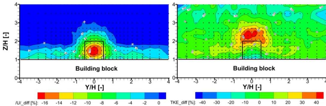
**Figure 4.** Distribution of the velocity-absolute value and turbulent kinetic energy difference between the reference case and the arrangement with the obstacle, relative to the initial state (in percent) in Plane 2.
