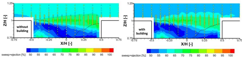
**Figure 6.** The proportion of sweep and ejection events at the lower part of Plane 3 measured without and with building. The colouring of the discrete measurement points refers to the dominant event according to the colour scheme as on Figure 5. Below the solid black line the proportion of out-of-range incoming hot-wire-probe samples (flow angle is larger than  $40^\circ$  or smaller than  $-40^\circ$ ) were larger than 5%
