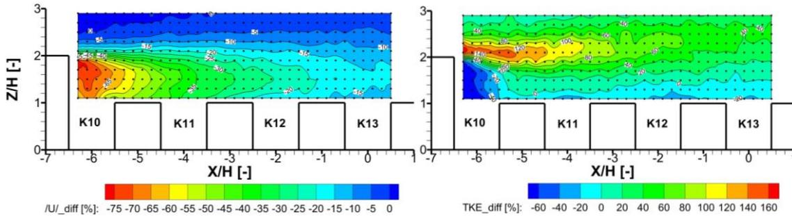
**Figure 3.** Distribution of the velocity-absolute value and turbulent kinetic energy difference between the reference case and the arrangement with the obstacle, relative to the initial state (in percent) in Plane 1
