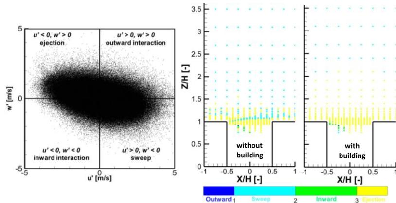
**Figure 5.** Left: Scheme of the quadrants and scatter plot of the measured velocity fluctuations in a point at  $Z/H=1.1$  (at  $X/H=0$ , without building). Right: distribution of the dominant event in a measurement points at K13 in Plane 3.
