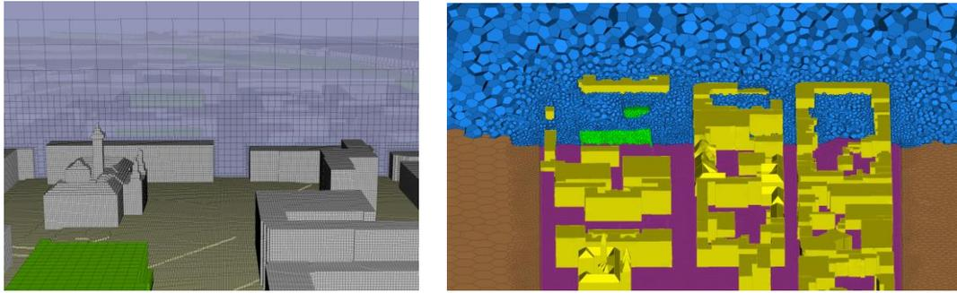
**Figure 3.** An overview of the meshes used in 3DAirQC: octree mesh generated by in-house multi thread Java code (left) and polyhedral mesh resulted from using ANSYS Fluent (right).
