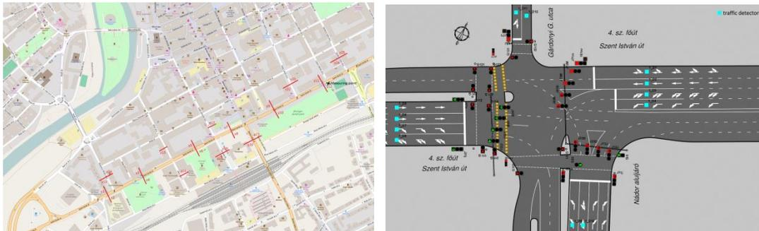
**Figure 4.** An overview of traffic sensor network of the city (on the courtesy of Hungarian National Roads Nonprofit Ltd. -Magyar Közút Nonprofit Zrt).
