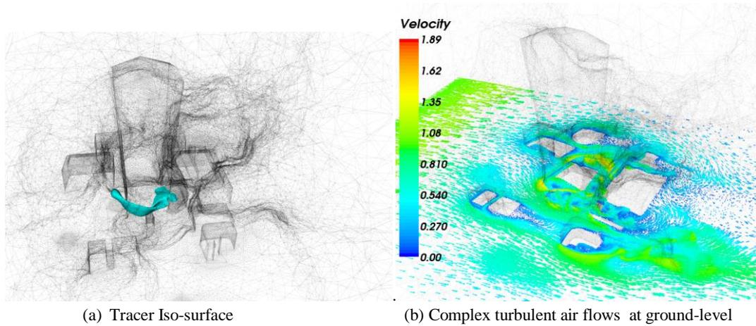
**Figure 5** Three-dimensional view of Adaptive mesh-refinement around the “Walkie-Talkie” building area, Central London together with: (a) a tracer isosurface and (b) the complex flow field near ground level.
