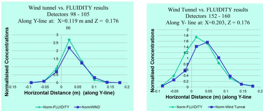
**Figure 4** Comparison of simulated normalised FLUIDITY tracer concentrations with wind tunnel measurements from the Enflo wind tunnel.
