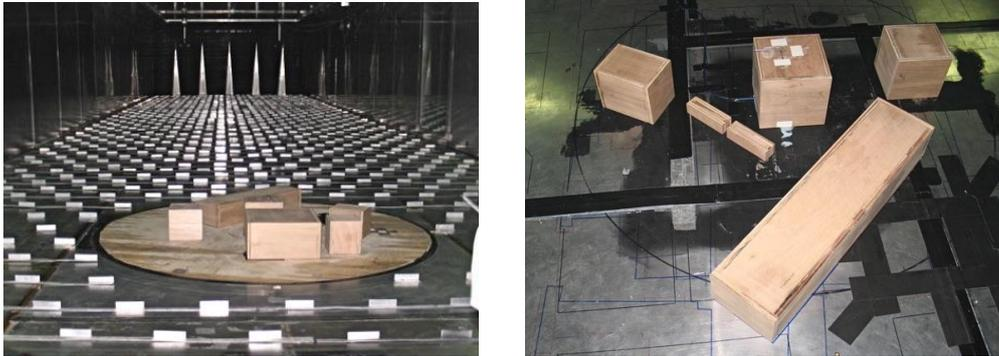
**Figure 1** The complex building configuration in the Enflo wind tunnel, University of Surrey, UK.
