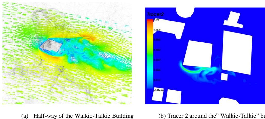
**Figure 6** Complex, turbulent flows and dispersion around the “Walkie-Talkie” building area at two different heights.
