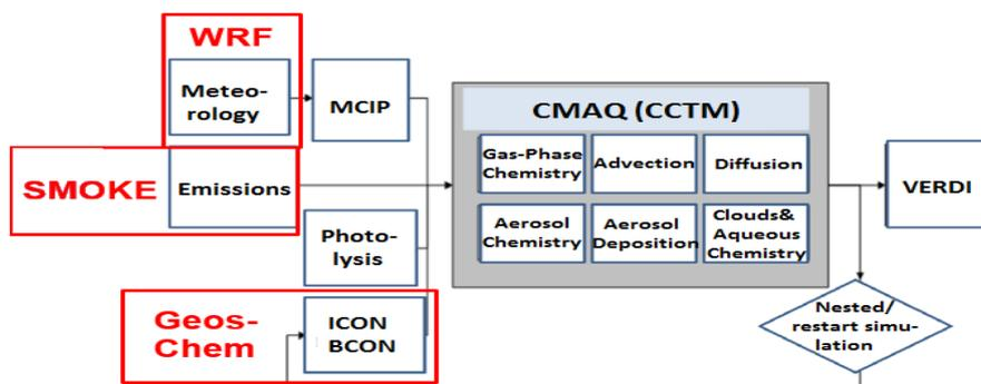
**Figure 2.** Sematic picture of the WRF – CMAQ – SMOKE model system. Black arrow shows the direction of the construction of the model system. Red box are optional model within the system, blue box is the sub processors in the CMAQ model
