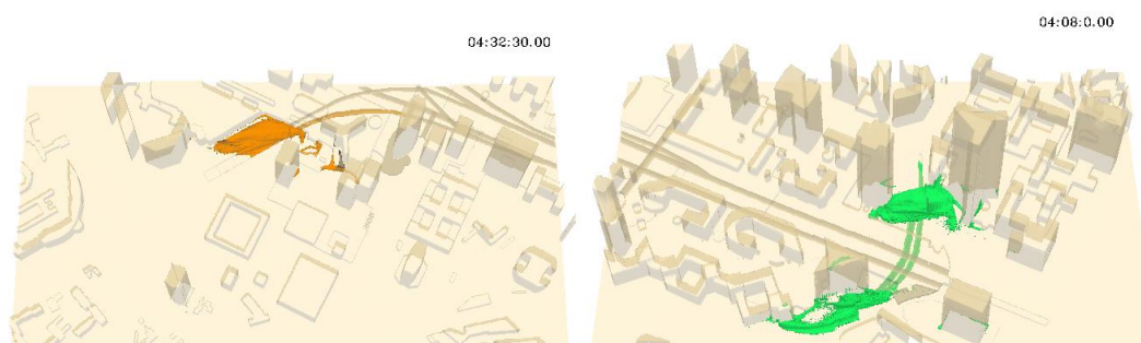
Figure 4. Left: South-West part of the calculation domain – Buildings and underground tunnels with opacity – Plume from orange release, time is 2’30’’ after the beginning of the emission – 3D iso-surface at 10 mg/m 3 in orange - Right: South-East part of the calculation domain – Buildings and underground tunnels with transparency – Plume from green release, time is 8’00’’ after the beginning of the emission – 3D isosurface at 2 mg/m 3 in green
