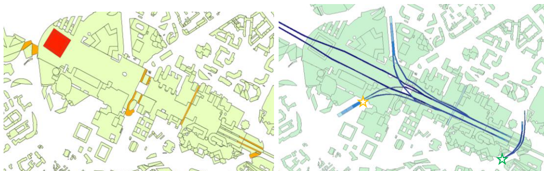
Figure 3. Left: Buildings footprints from BD TOPO® (IGN) in green and applied modifications to take into account arch structure (red) and aerial tunnels (orange). Right: Underground road tunnels in blue – Blue scale in giving the deepness of the tunnels floor – Orange and green stars show the location of considered hypothetical releases
