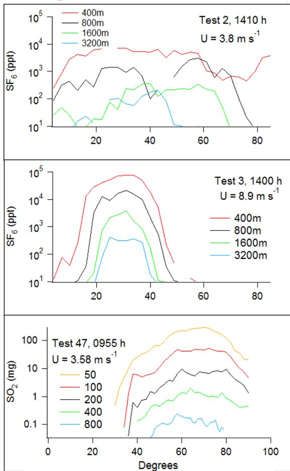
**Figure 2.** Tracer concentration plume cross-sections from PSB1 Tests 2 and 3 and PPG Test 47.
