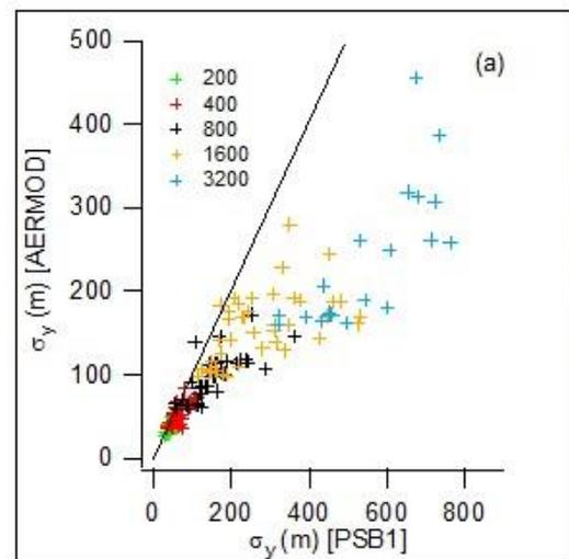
**Figure 1.** Plots of 10-minute period  $\sigma_y$  predicted by AERMOD versus those estimated from PSB1. The black line is the 1:1 reference.
