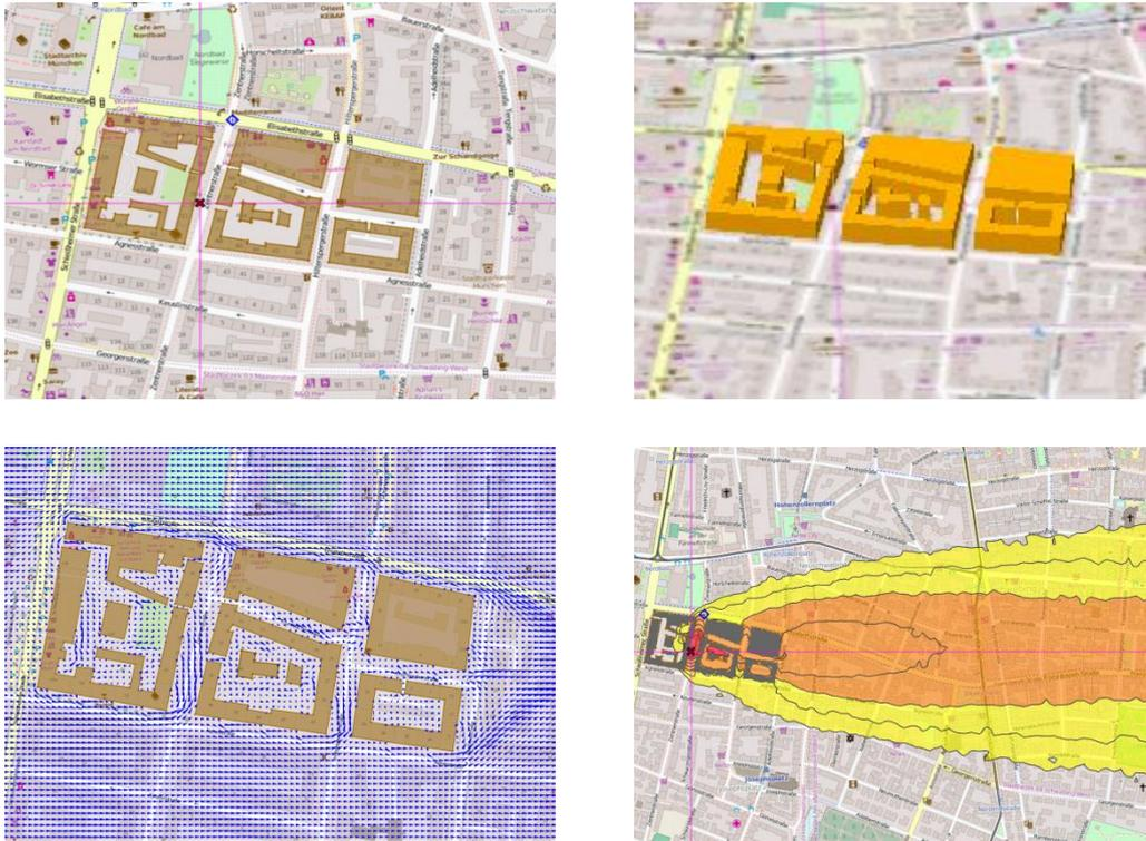
**Figure 2.** a, b, c, d. Scenario several building blocks. Figures show 2 d- and 3 d- sight (top left, top right), windfield (wind direction 270°) and inhalation dose for an arbitrary radionuclide and activity (bottom left, bottom right).
