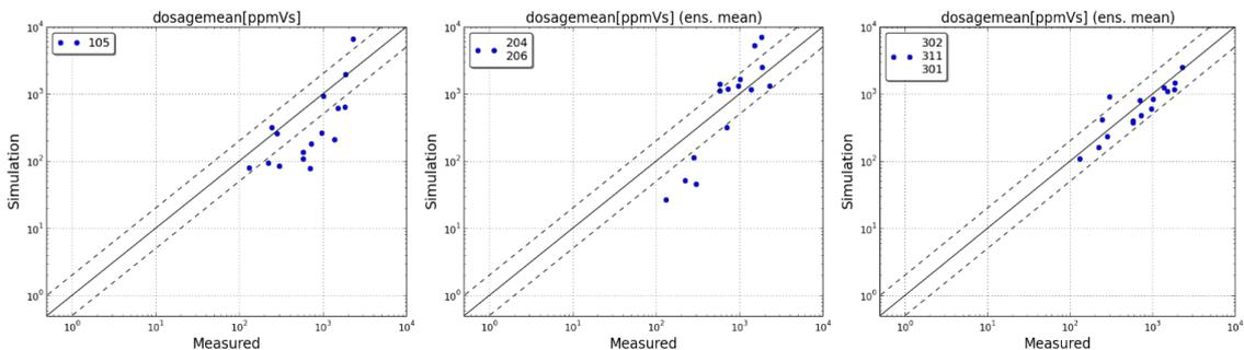
**Figure 2.** CUTE 3 test-case. Scatter-plots of measured versus ensemble averaged modelled mean dosage values at all receptors for all blind puff releases for model Type I (left), Type II (centre) and Type III (right).
