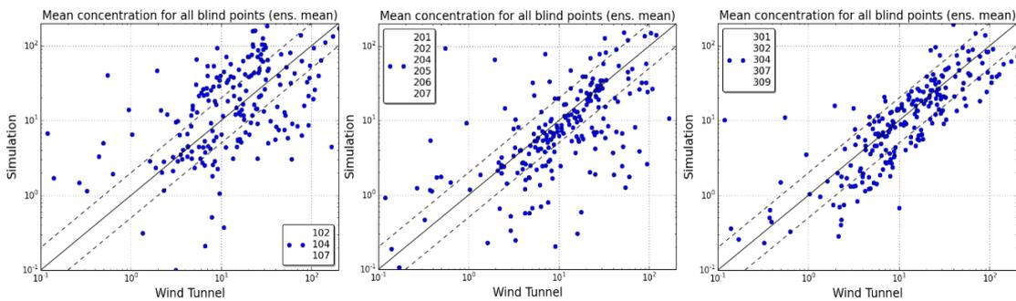
**Figure 1.** Michelstadt test-case. Scatter-plots of measured versus ensemble averaged modelled mean concentration values at all receptors for all blind continuous releases for model Type I (left), Type II (centre) and Type III (right).
