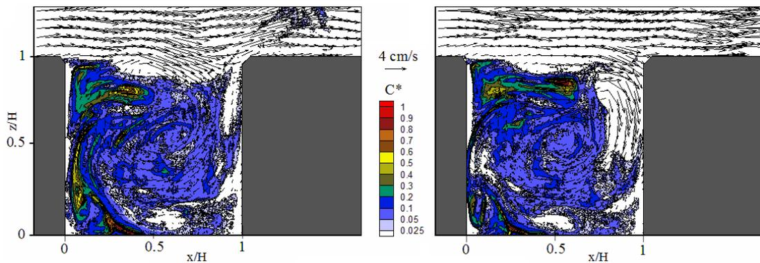
**Figure 4.** Maps of the instantaneous velocity (vectors) and concentration (colours) fields during the sweep mode. The right panel refers to the flow present 0.1 s later than that shown in the left panel.
