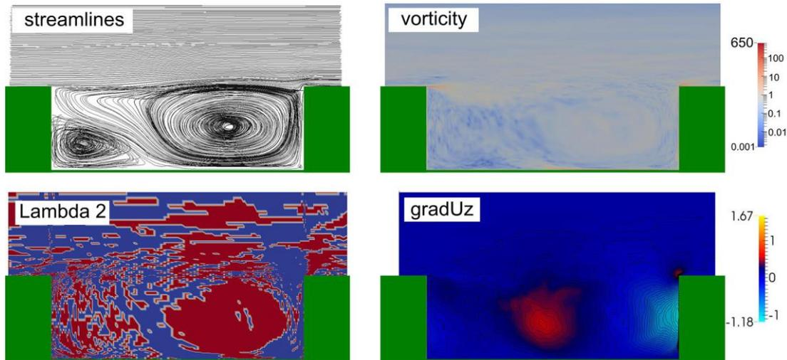
**Figure 3.** Application of vortex detection methods on the average velocity field of a street canyon with  $H/W = 1/3$
