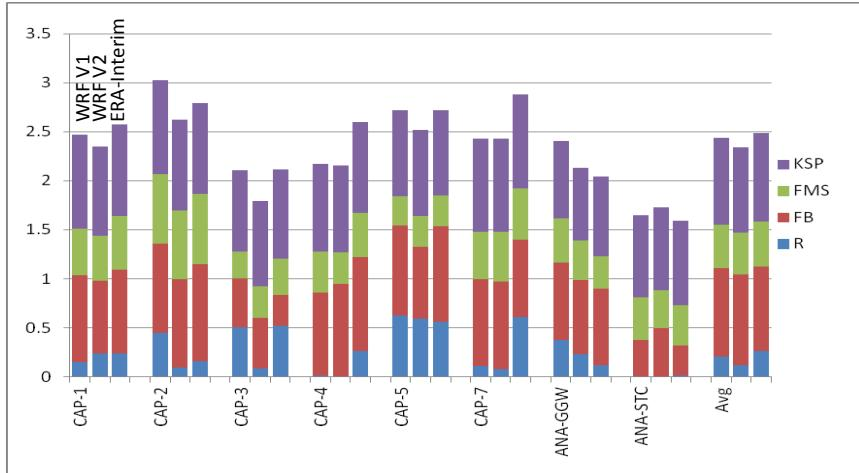
**Figure 1.** Bar plots of the normalised statistical parameters contributing to the rank as calculated in Eq. (1) for NAME driven by meteorological fields from WRF V1 (column 1), WRF V2 (column 2) and ERA-Interim (column 3).
