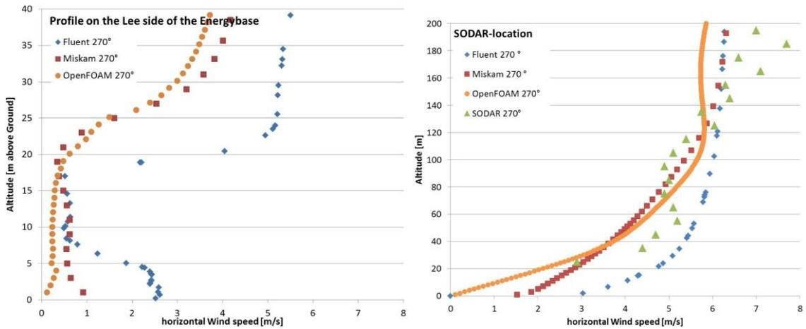
**Figure 7.** Profiles of the horizontal wind speed on the lee side of the building (left) and at the SODAR site (right) simulated with FLUENT, MISKAM and OpenFOAM for the 270 ° flow case compared to SODAR wind measurements averaged for a period with nearly homogeneous westerly flow (06.07.2015 from 7:00 am to 8:00 pm).
