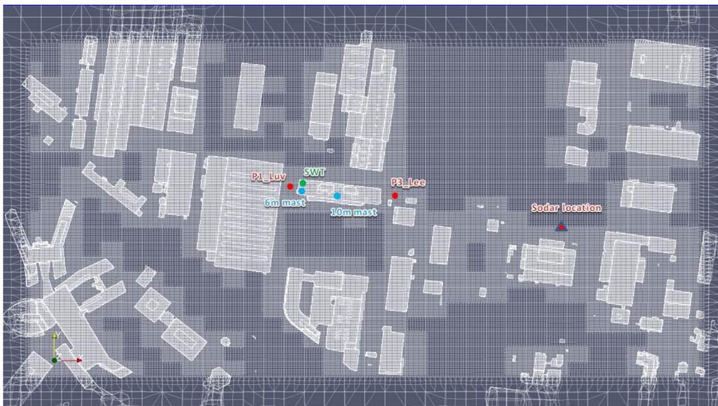
**Figure 5.** Mesh in OpenFOAM with ENERGY Base building in the centre of the model domain. Red points depict model grid points luv and lee of the building for model comparison (for 270° case), the red triangle indicates the SODAR site, green point the SWT site and blue points depict the 6m and 10m wind masts.
