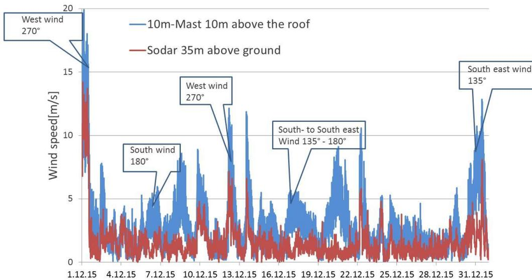
**Figure 4.** Time-series of SODAR wind speeds at 35m above ground and wind speeds measured with sonic at the 10m mast above roof for December 2015. The building is 25 m high. Main wind directions are depicted for selected episodes with good/poor agreement between the wind flow above roof and at the SODAR site.
