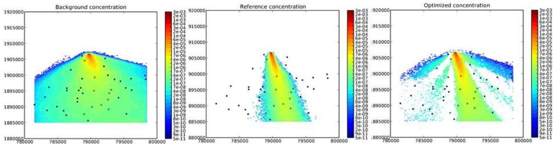
**Figure 2.** Spatial distribution of the *prior* (left), reference (middle) and optimized (right) concentrations (at the final time step) based on a configuration of the assimilation system using 60 members and 40 observation sites. The points represent the localization of the observation sites.
