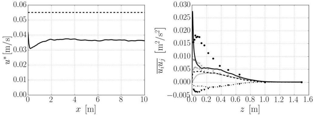
**Figure 3.** Left: friction velocity throughout the domain. Right: Reynolds stress profiles in the flat plate turbulent boundary layer simulation with synthetic turbulence inflow. Solid line:  $uu$ , dashed line:  $vv$ , dotted line:  $ww$ , dash-dotted line:  $uw$ . Symbols indicate the experimental values,  $\bullet$ :  $uu$ ,  $\times$ :  $vv$ ,  $+$ :  $ww$ ,  $\blacktriangledown$ :  $uw$ .
