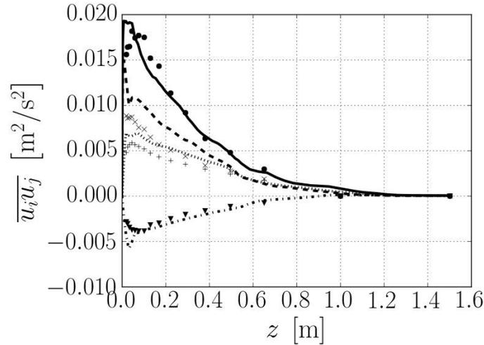
**Figure 5.** Reynolds stress profiles in the roughness boundary layer simulation with synthetic turbulence inflow. Solid line: uu, dashed line: vv, dotted line: ww, dash-dotted line: uw. Symbols indicate the experimental values, • : uu, × : vv, +: ww, ▼ : uw.
