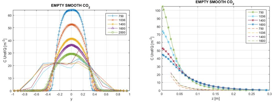
**Figure 2.** RANS2 using the MMK model cannot resolve the broadening of the plume in the way the experiment elucidates (left pane), but the right pane show that the gas is vertically dispersed in a way the experiment do not show. It is not clear if the concentration close to the floor was higher than the simulation but it is likely to assume that. Thus the density also is higher and maintained close to the surface.
