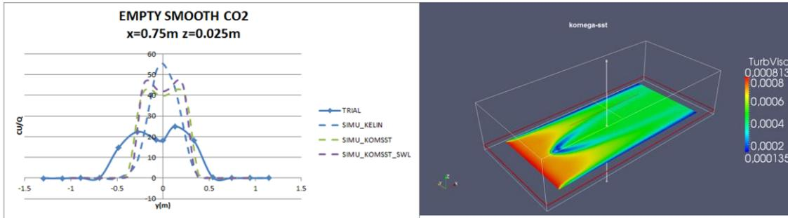
**Figure 4.** Normalized concentration close to the ground, effect of turbulence model. The left pane show the same pattern as Figure 3 that a modified turbulence model will improve the concentration profile but still cannot simulate the broadening of the plume.
