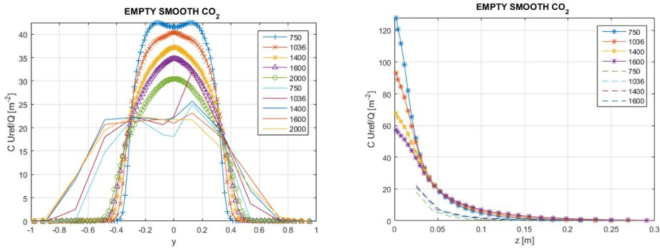
**Figure 3.** A minor correction of the MMK model is investigated in RANS2. By changing the Prandtl number in the GB formulation from unity to 0.714 a minor improvement is seen. The effect of the density gradient is increased. Still the left pane show unaltered broadening but a decrease of concentration levels and a double peak has emerged. The right panel indicate higher concentration close to the surface but the concentration levels are a factor of from the measured values.
