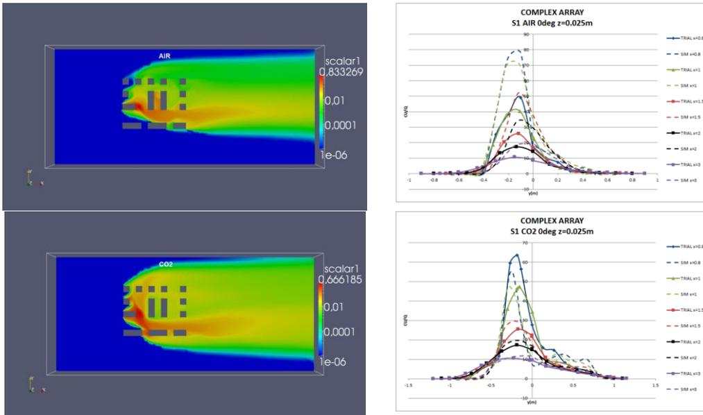
**Figure 6.** Mass Fraction contours for AIR (top) and CO<sub>2</sub> (bottom) and cross wind profiles close to the ground for the 0° orientated array
