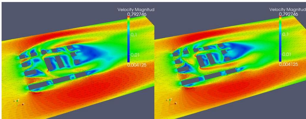
**Figure 5.** Velocity contours for AIR (left) and CO2 (right) for complex array case with Code Saturne
