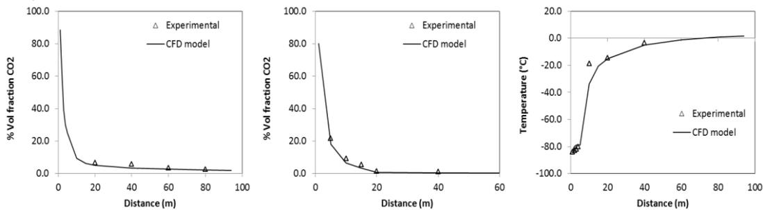
**Figure 3.** Concentration of CO<sub>2</sub> at 1m height from the ground along the axis of leak at different downwind distances from the source for T5DS1 (left) and T11DS1 (center) (sensors accuracy  $\pm 1\%$ ) - Temperature at 1m height from the ground along the axis of leak at different downwind distance from the source for T5DS1 (right)
