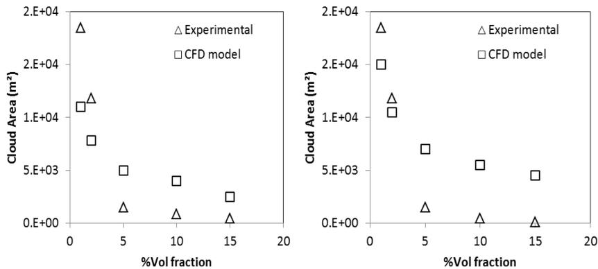
**Figure 2.** Comparison of surface area with experimental results at 50 secs (left) and at 190 secs (right) of BU5 case
