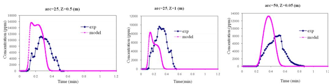
**Figure 6.** Concentration time series comparison plot for trial no 26
