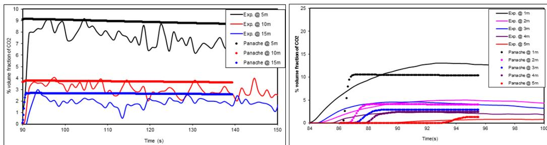
**Figure 4.** Temporal concentration of CO<sub>2</sub> at 1m height along the axis of leak at different downwind distances from the source for T8DS1 (left) and T14DS2 (right) (sensors accuracy  $\pm 1\%$ )
