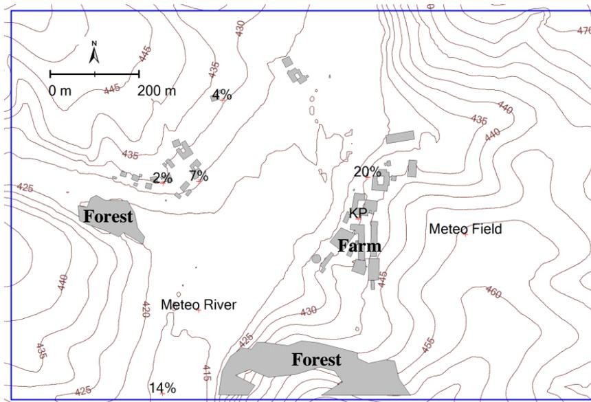
**Figure 1.** Model domain for dispersion modelling, orography, buildings, forests, and position of the meteorological stations as well as the inspection points for the panel field study. Numbers indicate the observed frequency of odour hours.
