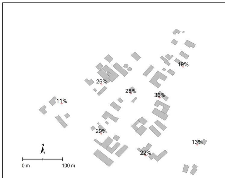
**Figure 2.** Model domain for dispersion modelling, buildings, and position of the inspection points for the panel field study. Numbers indicate the observed frequency of odour hours. The meteorological site was slightly outside the domain.
