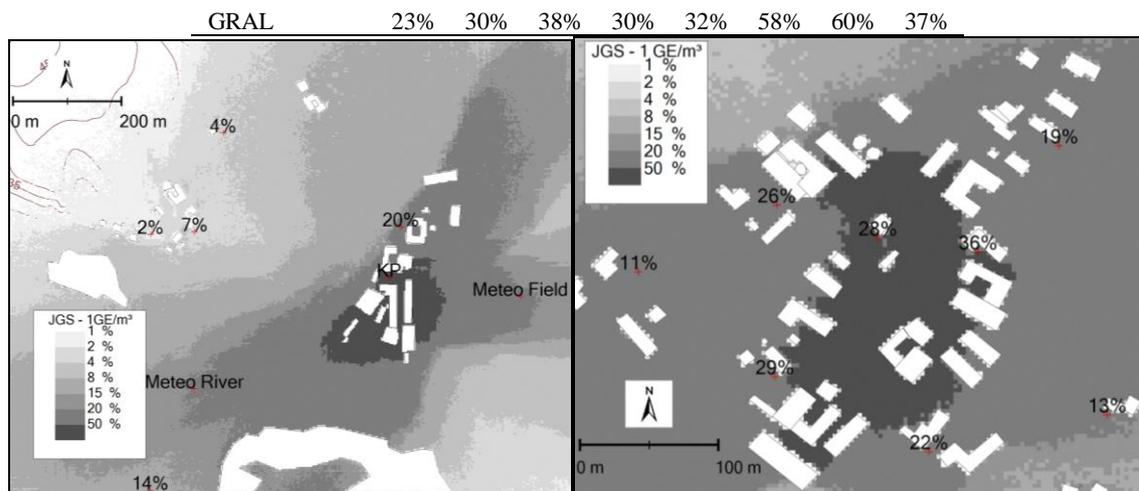
**Figure 3.** Simulated odour hour frequencies for data set A (left) and data set B (right). Odour threshold: 1 OU m<sup>-3</sup>
