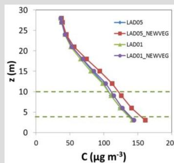
Fig. 4. Vertical profiles of spatially-averaged concentration within STREET A. Dashed lines indicate new trees location.
