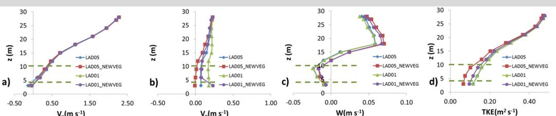
Fig. 6. Vertical profiles of average flow properties over the study street. a) wind speed normal to street (V<sub>n</sub>); b) wind speed parallel to street (V<sub>p</sub>); c) vertical wind speed (W); and d) turbulent kinetic energy (TKE). Dashed lines indicate new trees location.
